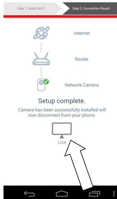
**10.** Setup is complete. The camera's **green** power LED & **orange** Internet LED should display **on**. You will see a live stream which you can view anytime you are connected to the Internet.
