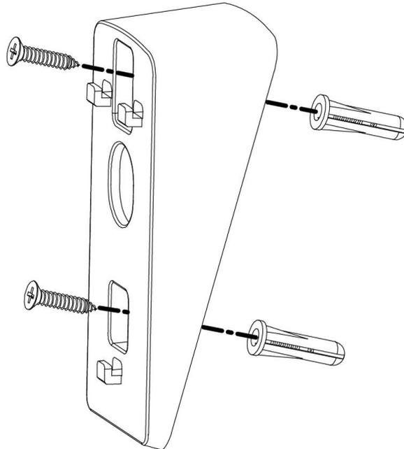
2. Attach the rear of the network camera to the mounting stand and tighten into place, as shown below:
